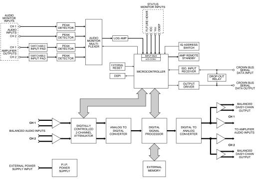
Fig. 5.1 IQ-P.I.P.-DSP Hardware Circuit Block Diagram
